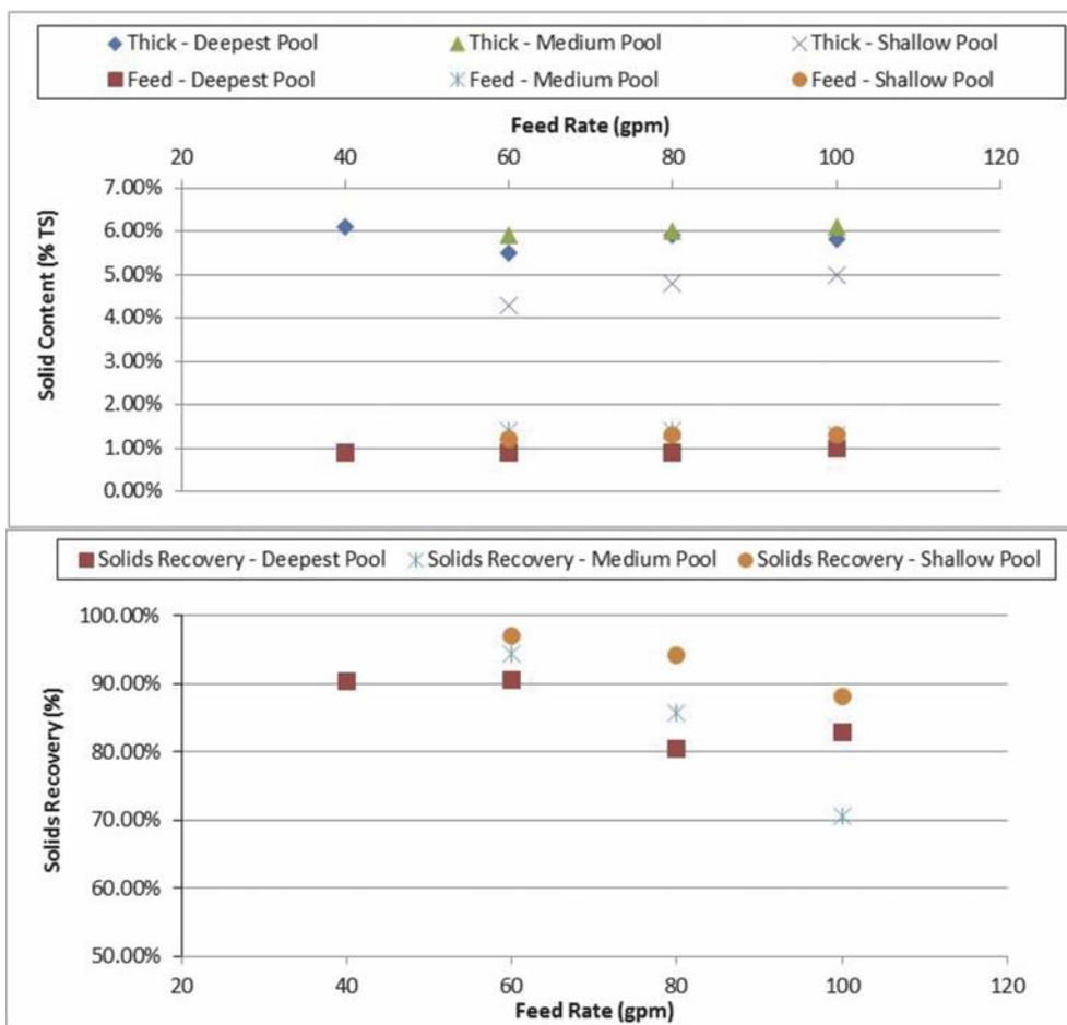
Figure 4. No-Polymer Operation, Medium Bowl Speed (2,590 rpm)
