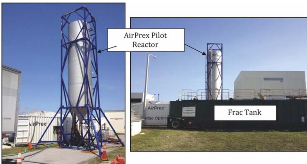
Figure 19. AirPrex Pilot and Frac Tank
