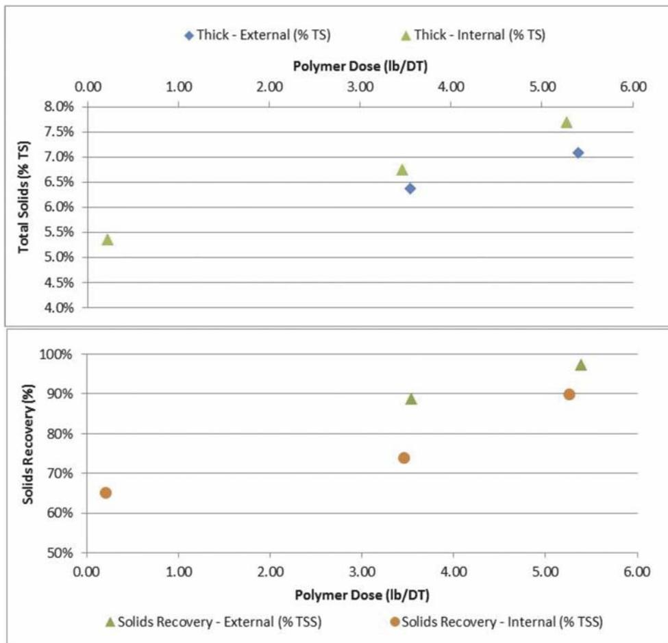
Figure 9. Dry Polymer: 150 gpm, Internal and External Injection, Medium Bowl Speed
