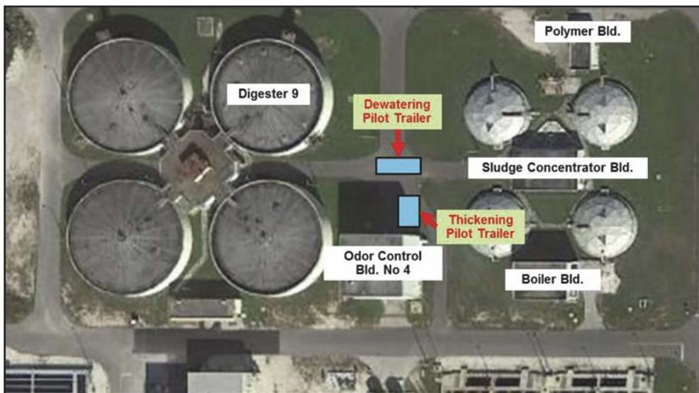
Figure 2. South District Wastewater Treatment Plant Pilot Site Plan Showing Centrifuge Installation
