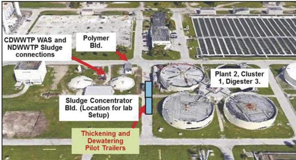
Figure 1. Central District Wastewater Treatment Plant Pilot Site Plan Showing Centrifuge Installation
