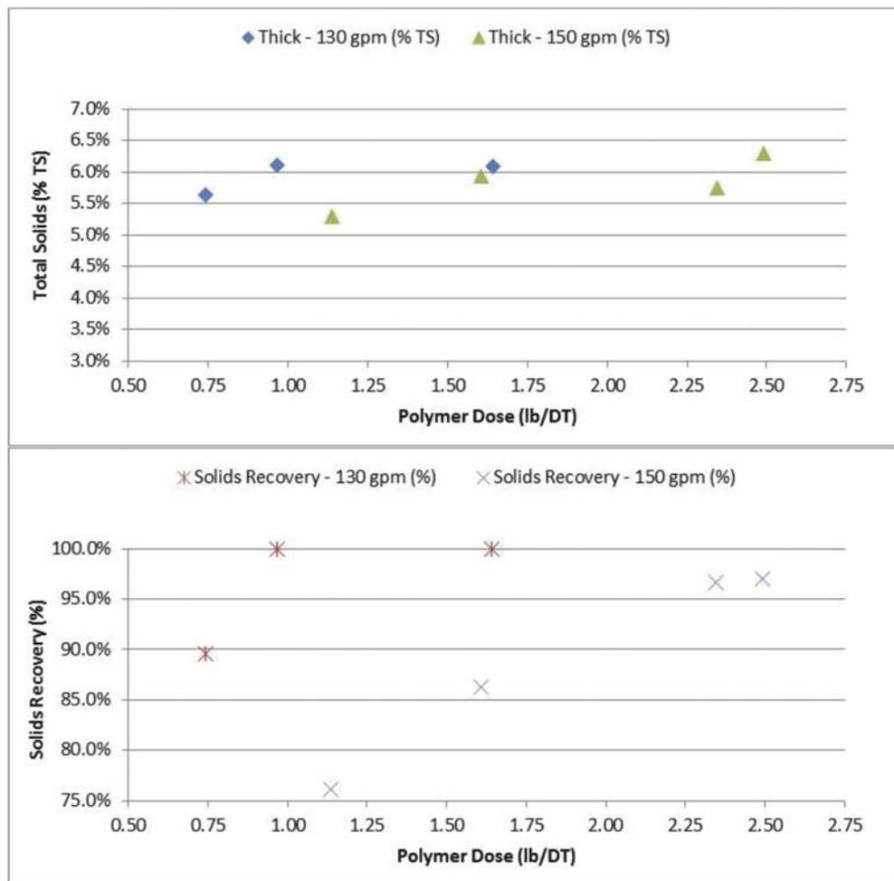
Figure 7. Emulsion Polymer: 130 and 150 gpm WAS Feed, Medium Bowl Speed
