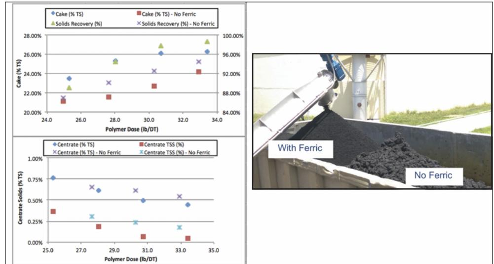
Figure 30. Central District Wastewater Treatment Plant Dewatering Polymer Curve Testing With and Without Ferric (data, left; photo of cake, right)
