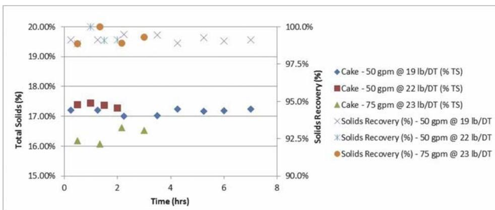
Figure 16. Extended Operation Using Dry Polymer
