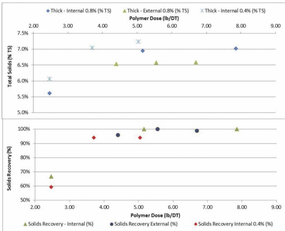
Figure 8. Dry Polymer: 130 gpm WAS Feed, Internal and External Injection, Medium Bowl Speed
