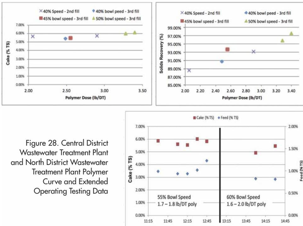
Figure 28. Central District Wastewater Treatment Plant and North District Wastewater Treatment Plant Polymer Curve and Extended Operating Testing Data
