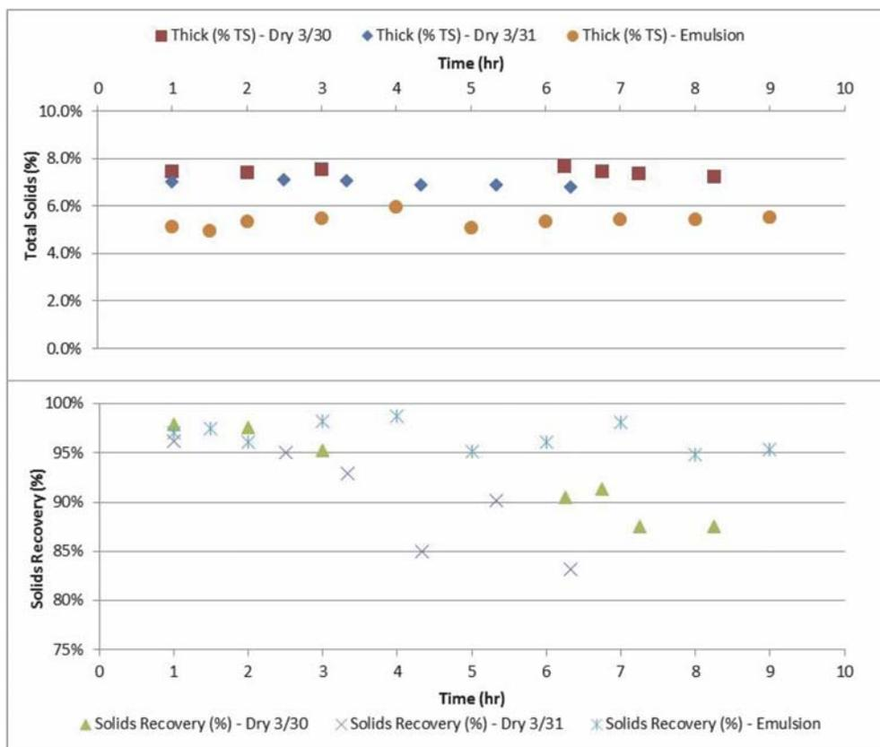
Figure 10. Extended Thickening Operation at 135 gpm
