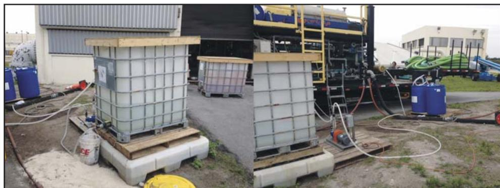
Figure 6. Temporary Dry Polymer Setup
