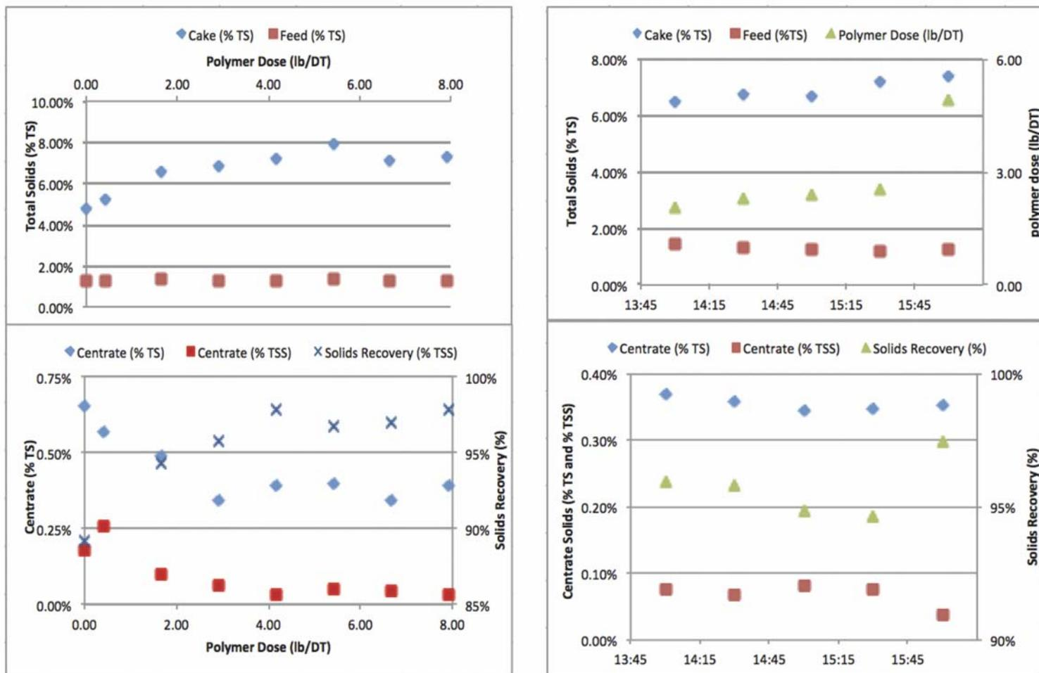
Figure 25. Dry Polymer Curve and Extended Operation Data, Central District Wastewater Treatment Plant, Waste Activated Sludge Only
