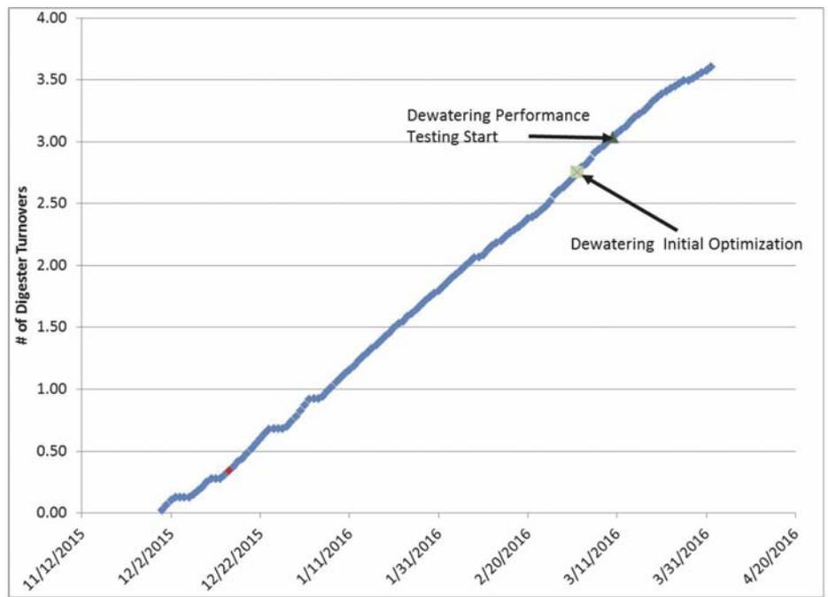
Figure 13. Digester 9 Turnover Progress During Phase 2 Operation
