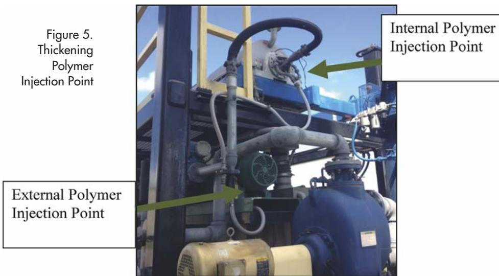
K144-L, which is a cationic, high-molecular-weight emulsion polymer. Polymer dosage, using internal injection, was slowly increased at a constant throughput of 100 gpm, while visually monitoring the clarity of the centrate. The testing was conducted at the shallowest pool depth and a differential speed of 12 rpm. Once
