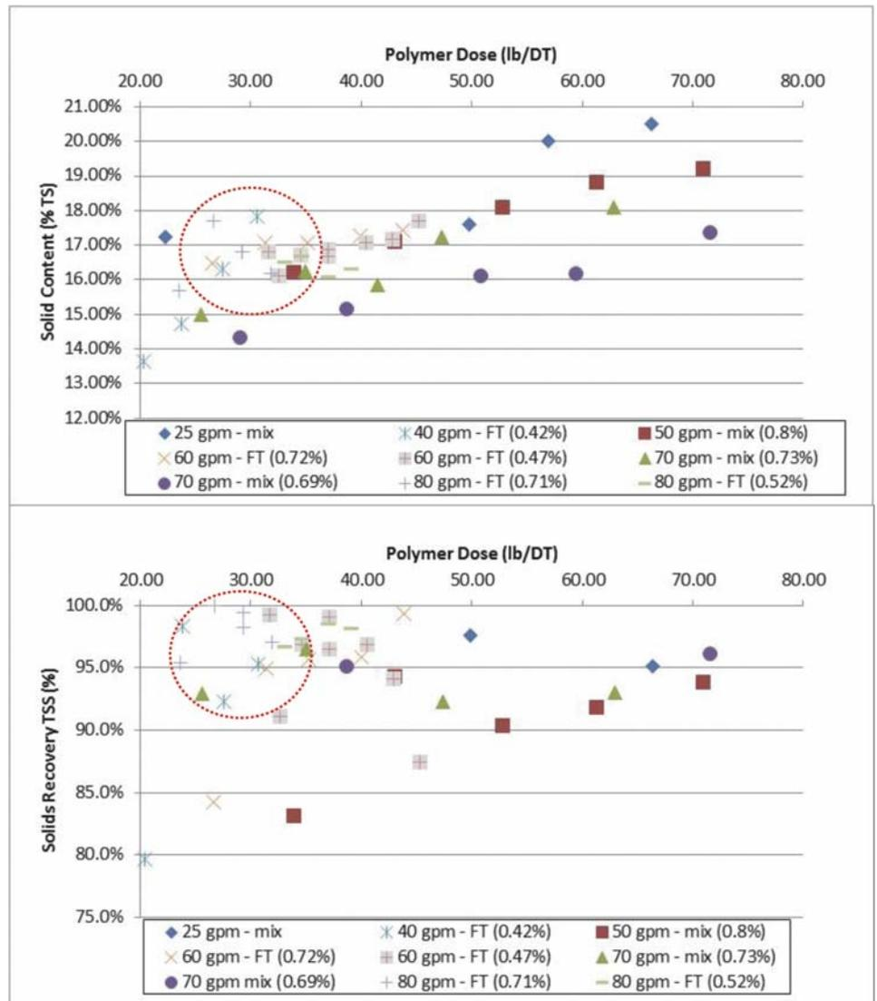
Figure 14. Compiled Dry Polymer Curves from Digester 9
