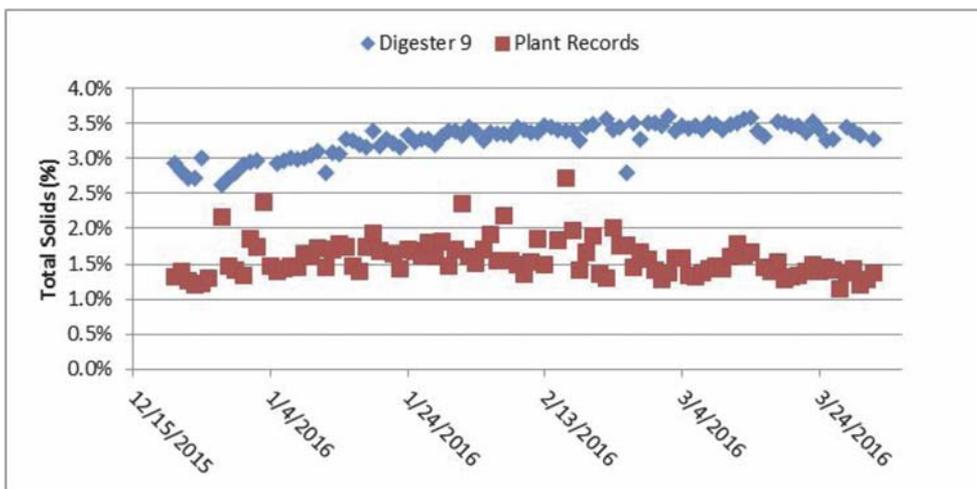
Figure 12. Digester Concentration Comparison, Digester 9 Versus Plant Records
