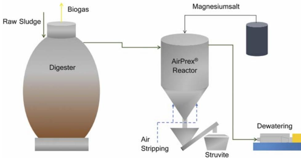
Figure 18. Typical AirPrex Process Flow Diagram (Courtesy of CNP Corp.)
