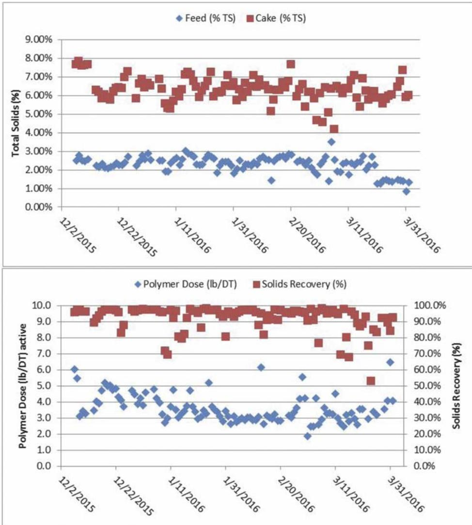
Figure 11. Phase 2 Continuous Thickening Operation
